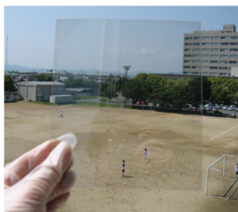
Transparency of FTO on a glass substrate
